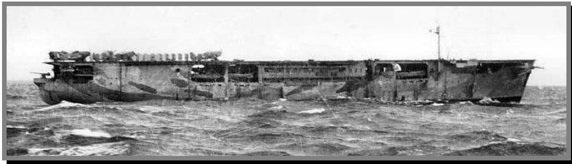
HMS Audacity with Martlets on her flight deck. Note she had no hanger so the aircraft were open to the elements
